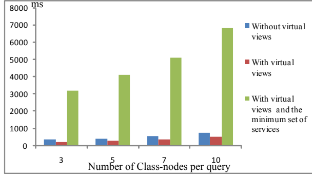
Figure-6: The response time of the mashup system before and after introducing the virtual layer and when the minimum set of services algorithm is applied
